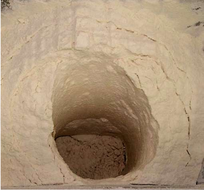
Fig. 1: An example of unreliable flow of a cohesive powder.
