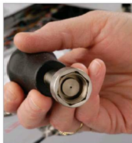
Septum nut remains in tool until reinstalled.
