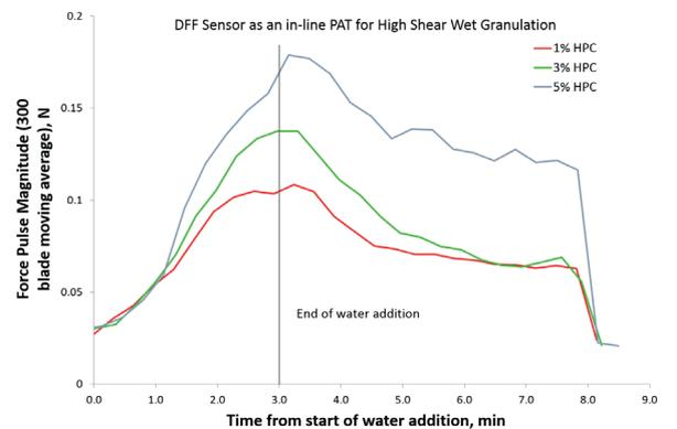
The principal output of the Drag Force Flow sensor for powder mixing applications, including granulation, is the Force Pulse Magnitude (FPM). FPM is the difference between the force at maximum and the preceding minimum. Each FPM, therefore, characterises a passing of one blade under the probe pin. Being a differential measurement, FPM provides a reliable characteristic of the wet mass consistency and densification, since it is independent from possible zero drift in the raw signal.
