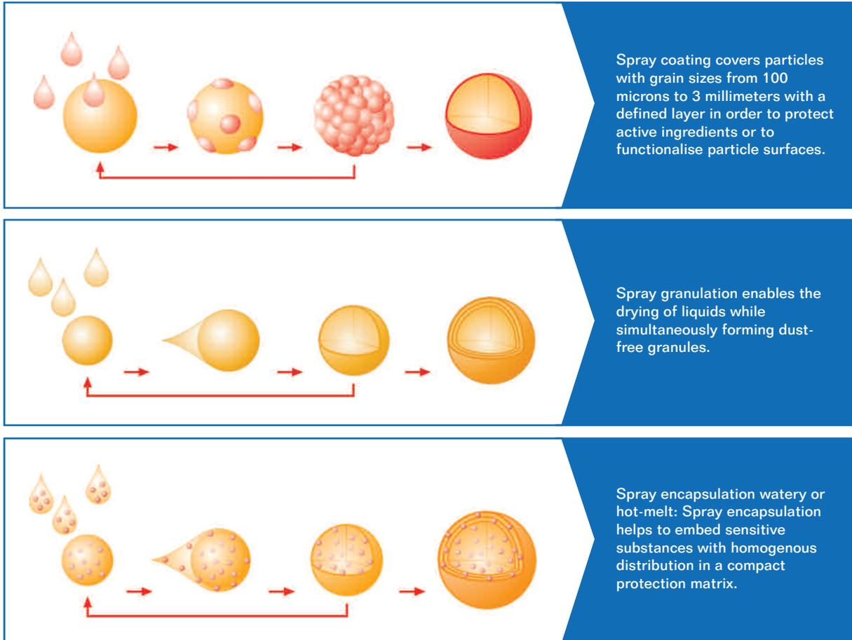
Spray coating covers particles with grain sizes from 100 microns to 3 millimeters with a defined layer in order to protect active ingredients or to functionalise particle surfaces.
