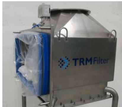
FIGURE 3: Bag-in/Bag-out filter replacement
