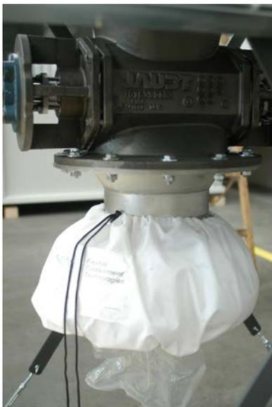
FIGURE 5: Dust collection in continuous foils
