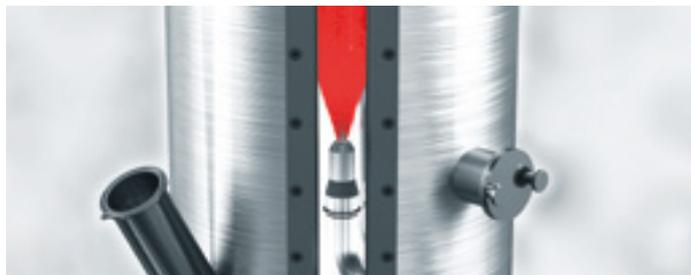
**Figure 4:** The pulsating gas flow, in contrast to the continuous gas flow, due to the high degree of turbulence no temperature and speed gradients. Therefore all particles experience the same thermal treatment.
