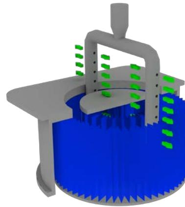
PICTURE 3: Vertical rotating nozzle fork eases dust removal
