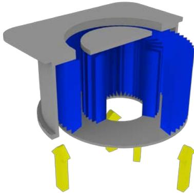
PICTURE 2: Airflow through the filter cartridge
