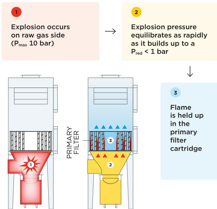
PICTURE 9: Internal pressure diversion with ECH and ECR Dust Collectors
