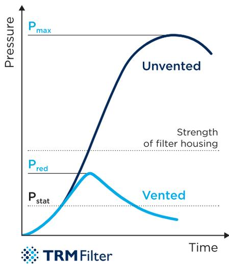
PICTURE 5: Explosion pressure curve
