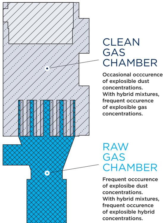
PICTURE 3: Frequency of occurrence of explosive concentrations in the chambers of dedusting filters
