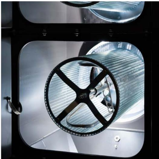
PICTURE 1: Rotatronic filter cleaning in the filter cartridge
