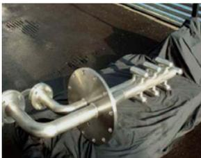
Insertion pipes with two-substance nozzles
