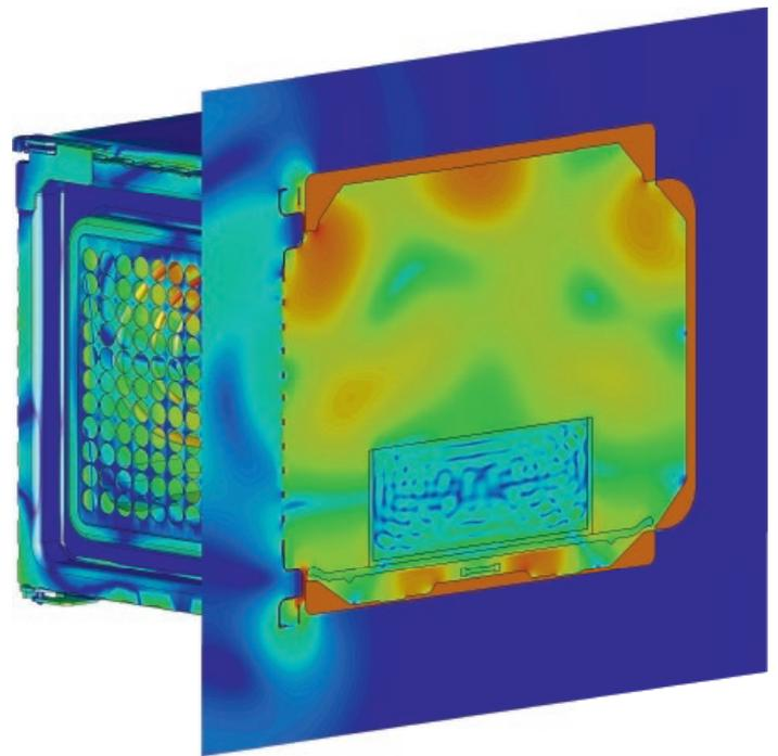
Figure 1 Leakage from a poorly shielded oven.
