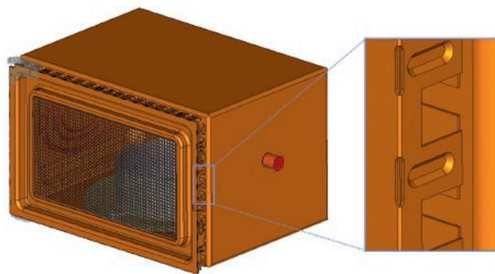
Figure 5 Door fins (highlighted) in a microwave oven.
