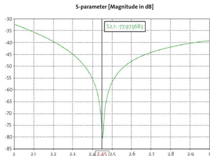
Figure 8 S-parameters of the optimized door fins.
