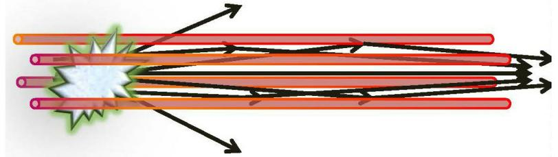
Typical fibers consist of a transparent glass core surrounded by a cladding material with a lower index of refraction. When light tries to leave the core, it gets reflected back inward. But solid optical fibers can only handle so much power, and they need physical support that may not be available where the cables need to go, such as the upper atmosphere. Now, Milchberg's team has found a way to make air behave like an optical fiber, guiding light beams over long distances without loss of power.
