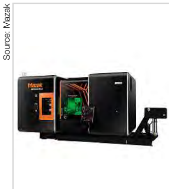
I-400 AM integrates direct energy deposition AM technology into a 5-axis multi-tasking machine.
