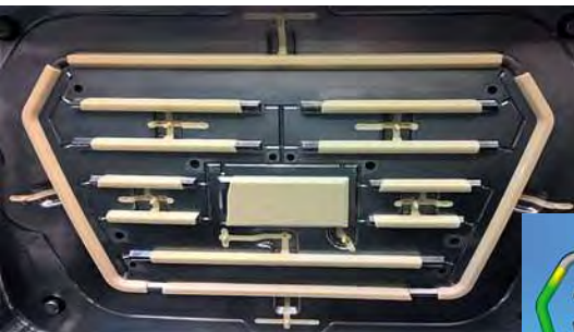
Comparison between real moulding and FLEXflow simulation. Flow balancing predictivity matches reality perfectly.
