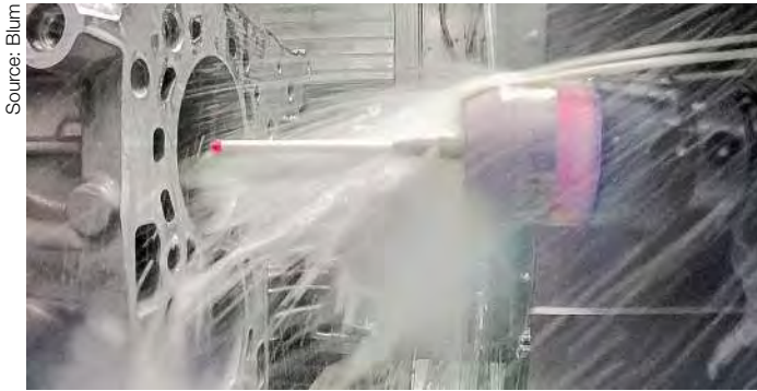
Pulling measurements of grooves and bars can be carried out with the TC61 touch probe system as well.
