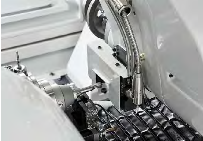
Anca's Laser Plus provides a robust measurement solution with quick measurement times which will not significantly add to the grinding cycle time.
