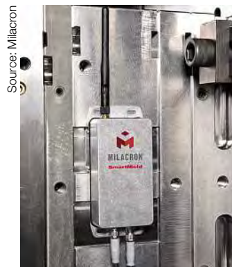
Smart-Mold sends and receives information from other equipment to optimise the cell performance.
