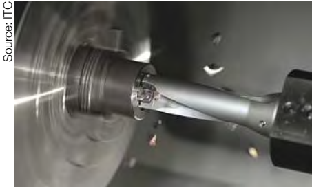
Two different geometries are offered for drilling steel, stainless steel and cast iron.
