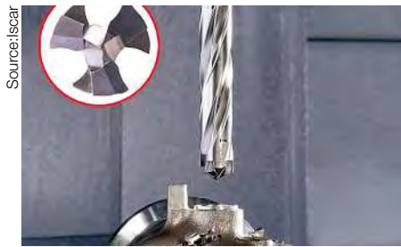
Sumo-3-Cham's geometry shapes the produced chips optimally.
