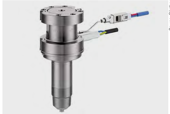
The two-part shaft in Günther hot runner nozzles offers optimum thermal separation from the mould. The shaft, which is made of two different materials, prevents uncontrolled thermal dissipation and allows for the best possible thermal separation between the mould and the nozzle.
