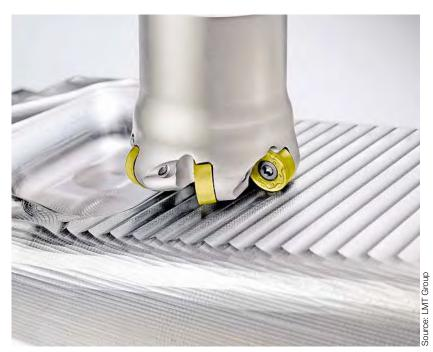
The roughing inserts of the Acu-Jet Double 6 Premium can be used up to 12 times.
