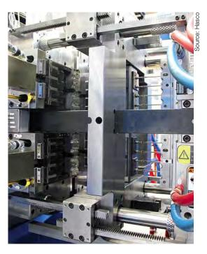
The photo shows a stack mould with a spinstack inside
