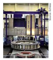
The multitasking-machine "Vertimaster" is available in several sizes and configurations.
