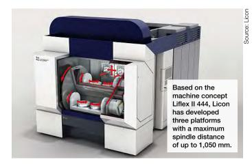
crease the manufacturing output of housings for passenger car steering systems, a concept was realised to enable the machining of two workpieces per spindle simultaneously. The advantage thus for the two-piece clamping is the corresponding machining of two
